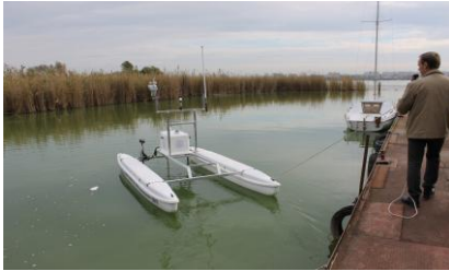
Autonomous naval surface platform for the acquisition and transmission of data from a maritime district Project PSCD of MOfD 151/2016
