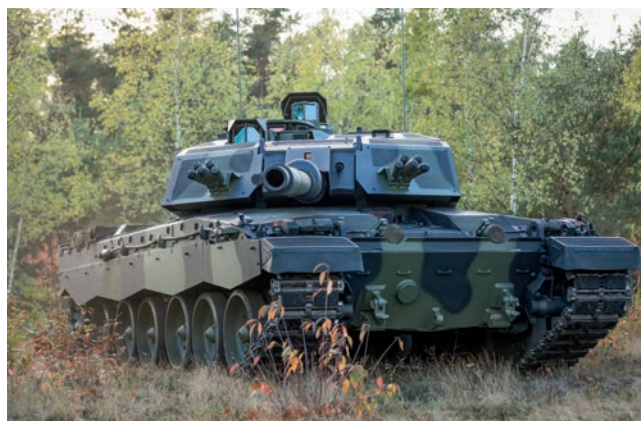
120 mm L55A1 operated by Challenger MBT
