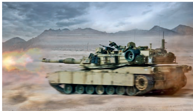
120 mm M256 (license from L44) operated by M1A1/A2 Abrams MBT
